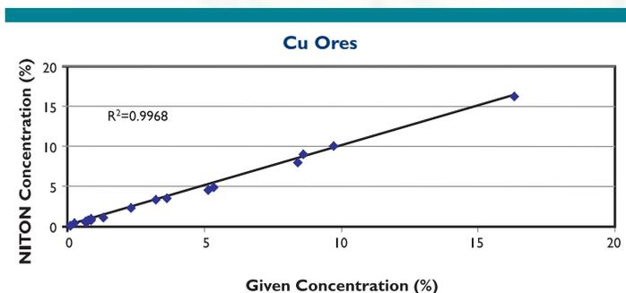
Correlation for Cu Ores using data generated from an XLt 500 compared to concentrations obtained from a conventional laboratory method like AA (Atomic Absorption). The correlation shows that the NITON portable analyzer can provide laboratory quality results on-site in seconds.
