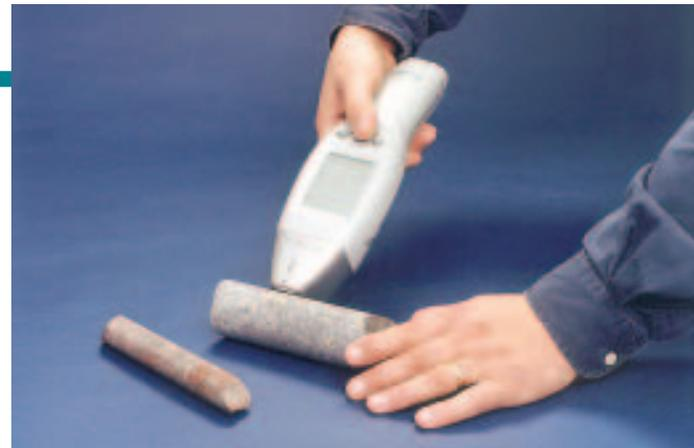
The **XLt 500 Series analyzer** offers the user the speed and efficiency of x-ray tube excitation, while greatly reducing the regulatory demands typically encountered with isotope based units. The XLt can be easily shipped from state to state and between most countries with minimal paperwork and expense.
