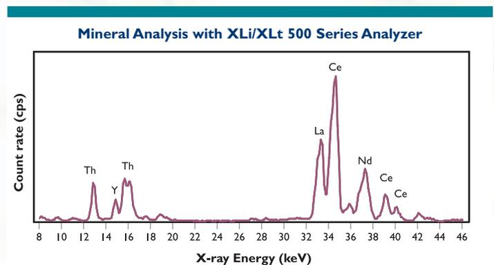
Qualitative spectrum generated using an XLi 500 and NITON Data Transfer (NDT) software for a monazite ore sample. In addition to a complete quantitative analysis of up to 25 elements, the analyzer also generates and stores a qualitative spectrum for each analyzed sample. This allows for quick and simple peak identification and report generation.
